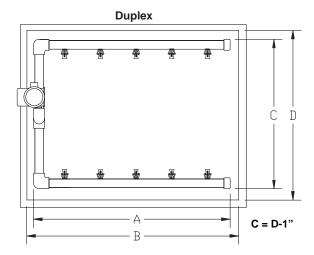
Introduction: Eductors utilize a unique venturi design which enables smaller pumps to circulate larger volumes of tank solution. The eductor can circulate four to five gallons of solution for each gallon pumped.
